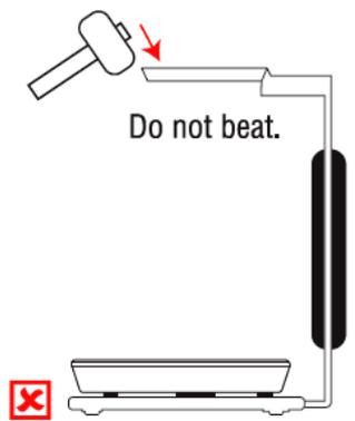
The upper scale cup holder must not be pressed by hand or lifted directly, not to be impacted.
