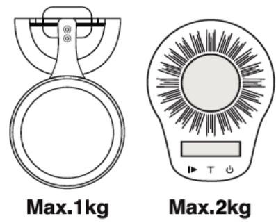
The maximum load of a coffee scale is: 1 kg on the upper scale and 2 kg on the lower scale. Because the upper scale is a floating design, it cannot achieve over-loading protection, so when it is hit by more than 2 kg, it will cause Err2 damage.
