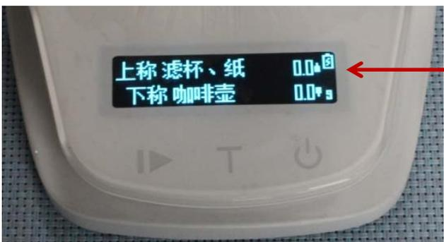
The charging symbol must be displayed when charging. In order to protect the battery life, it takes about 4 hours to fully charge with a small current. It can still be used in charging.
