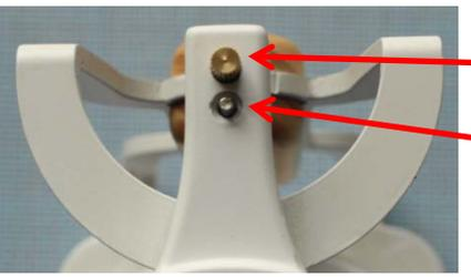
1. Loosen the copper nut, remove the cup holder, and replace the copper nut .
